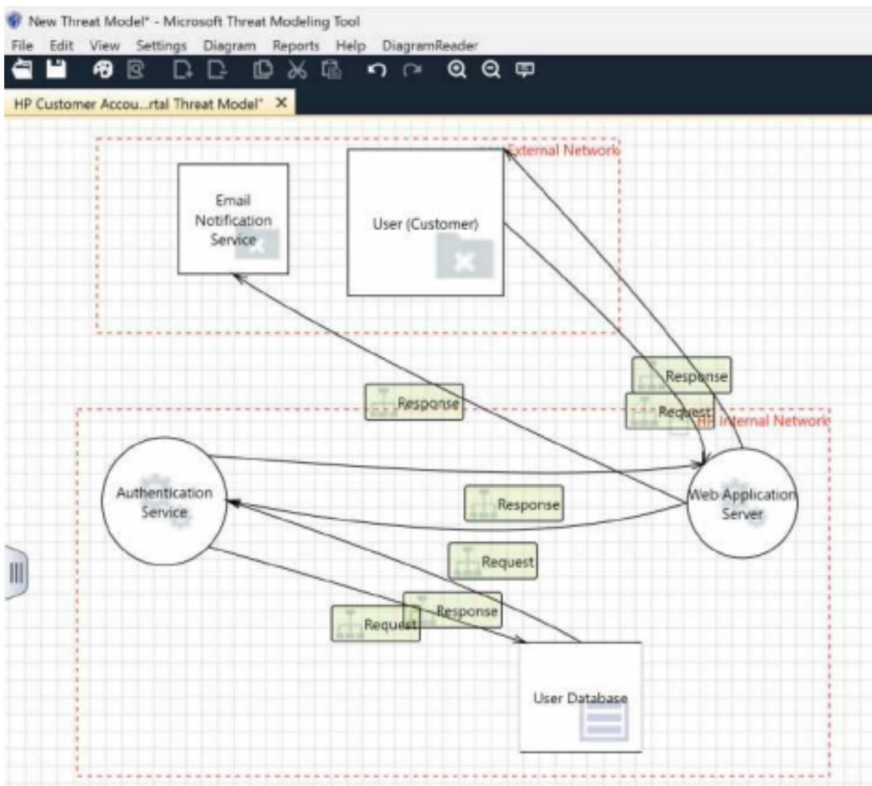
Using the Microsoft Threat Modeling Tool (MTMT), two trust boundaries were defined: one external and one internal. The system includes a user, web app, authentication, database, and email components. MTMT identified multiple STRIDE-based threats, primarily related to spoofing, tampering, and information disclosure across trust boundaries. Key mitigations include enforcing HTTPS with HSTS, implementing MFA, encrypting all sensitive data, and applying RBAC with least privilege.
